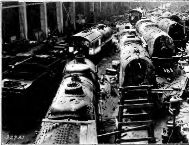
FIG. 33. REBUILDING CONSOLIDATION ENGINES IN LOCOMOTIVE REPAIR SHOP
